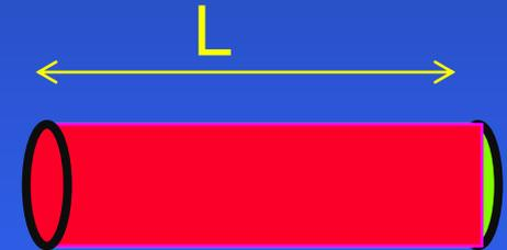
$$\left. \begin{array}{l} \text{Take : } \sigma = 7.94 \cdot 10^{-30} \text{ m}^2 \\ n_e = 10^{20} \text{ m}^{-3} \\ L = 1 \text{ cm} = 10^{-2} \text{ m} \end{array} \right\} \longrightarrow F_{\text{scat}} = 10^{-11}$$
