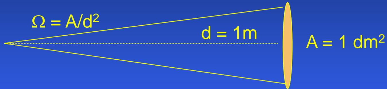
$$\left. \begin{array}{l} \Omega = A/d^2 = 10^{-2}\text{sr} \\ \text{Solid angle fraction } \chi = \Omega/(4\pi) = 10^{-3} \end{array} \right\} \longrightarrow F_{\text{coll}} = 10^{-3}$$
