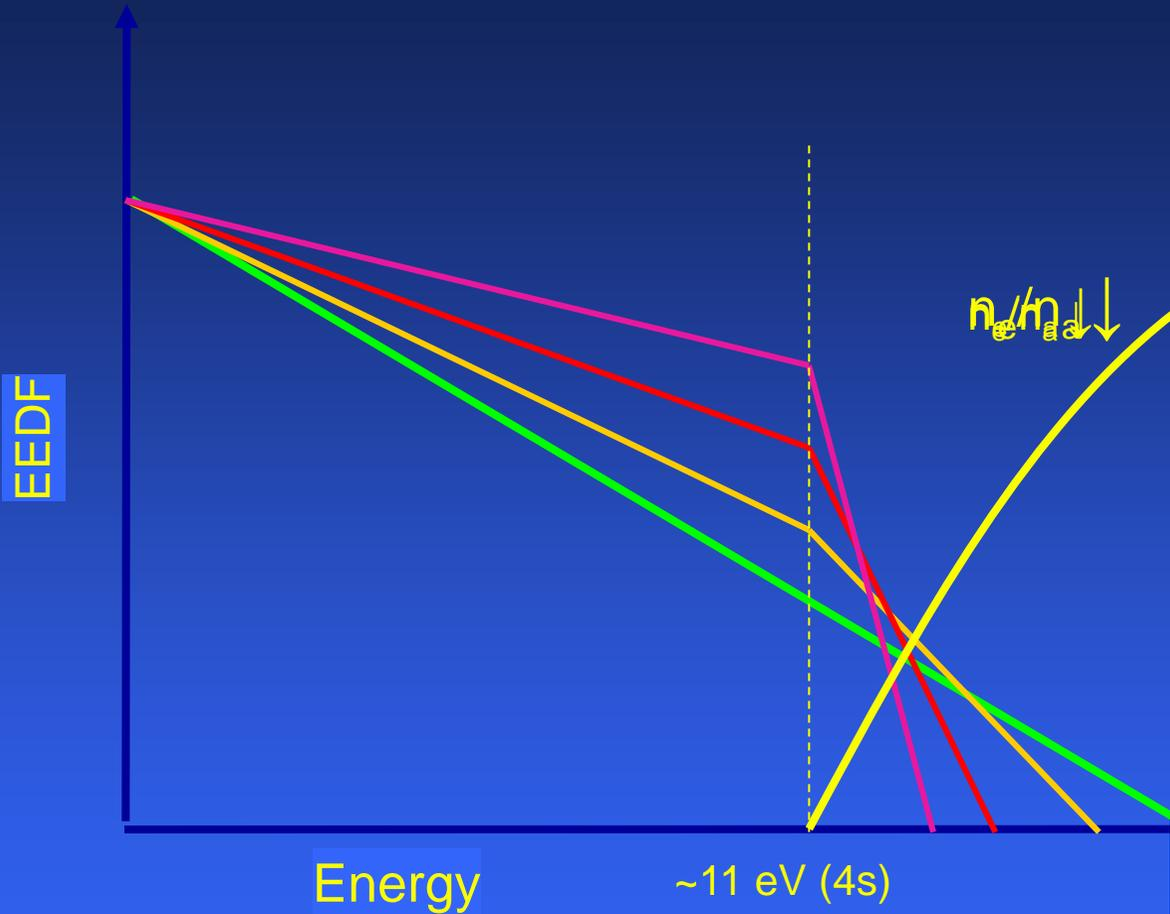
An EEDF with broken tail needs a higher mean-E
